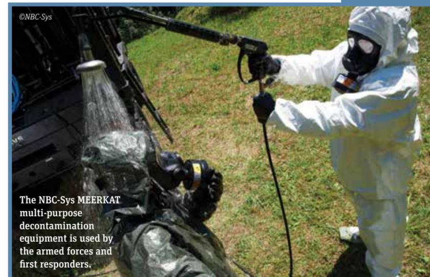
The NBC-Sys MEERKAT multi-purpose decontamination equipment is used by the armed forces and first responders.
