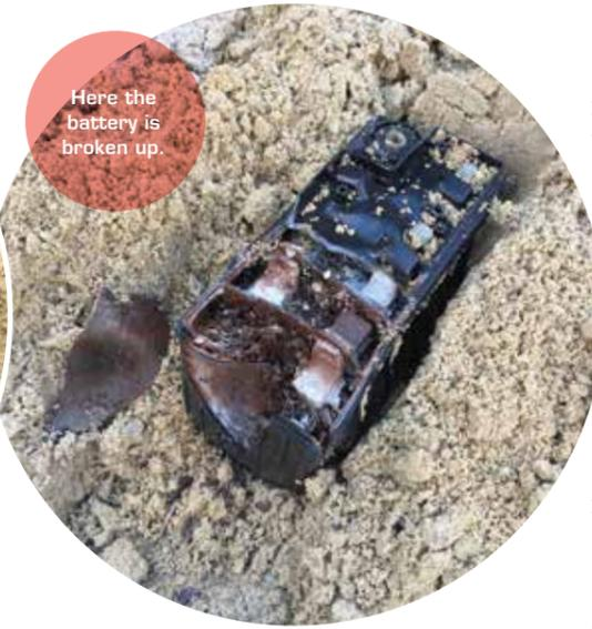
Here the battery is broken up.
